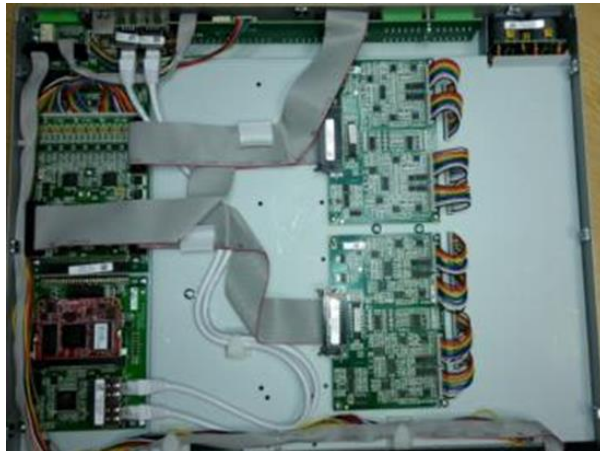
8 channel with Dante card fitted
