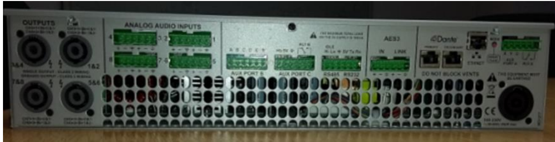
4 channel with Dante card fitted
