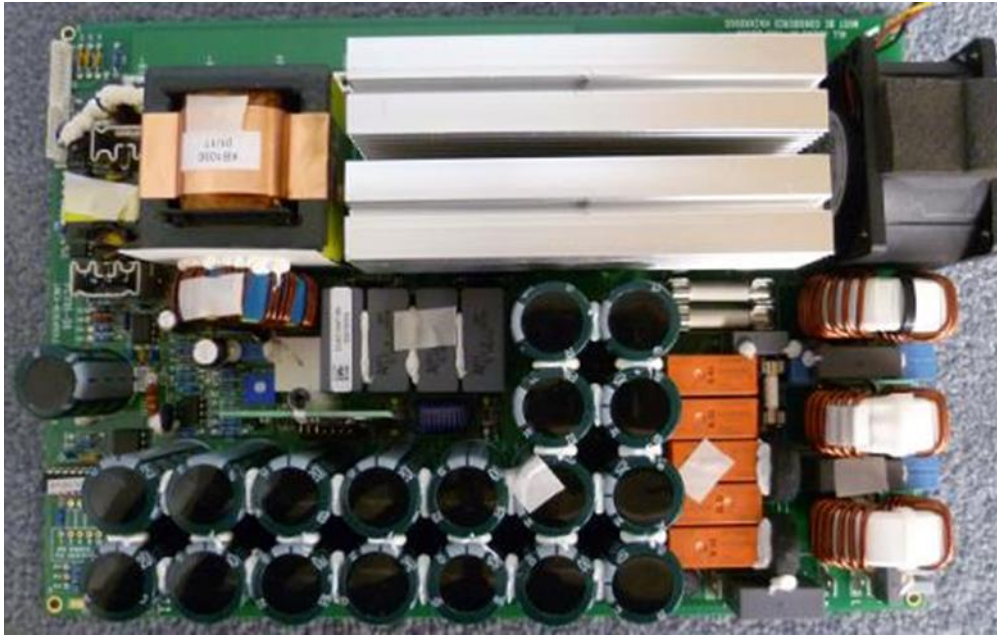
Power supply PCB print side
