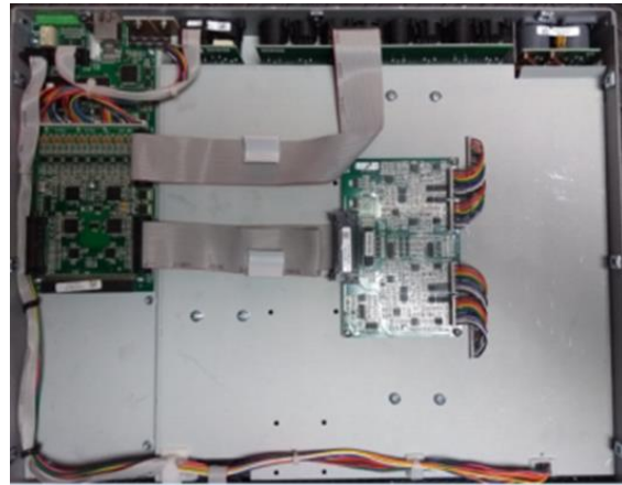
4 channel without Dante card fitted
